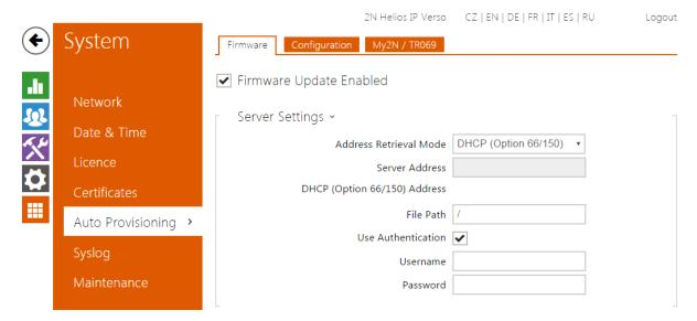
The **2N Helios IP** intercoms help you update firmware and configuration manually, or automatically from a storage on a TFTP/HTTP server selected by you according to predefined rules.
