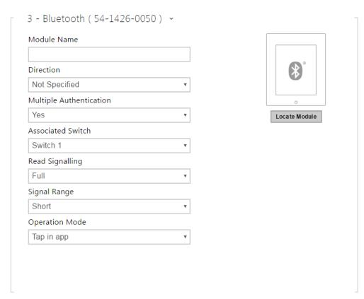
• Module name - set the module name for logging events from the Bluetooth module.
