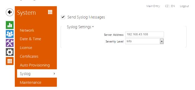
The **2N Helios IP** intercoms allow you to send system messages to the Syslog server including relevant information on the device states and processes for recording, analysis and audit. It is unnecessary to configure this service for common intercom operation.
