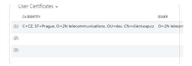
Press to load a certificate saved on your PC. Select the certificate (or private key) file in the dialogue window and push **Load**. Press to remove a certificate from the intercom.
