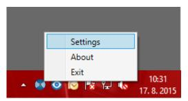
2. Set up the COM port for the connected reader.
