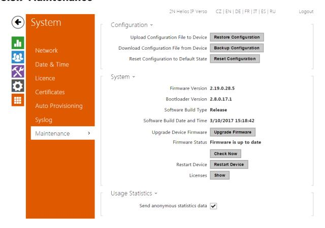
Use this menu to maintain your intercom configuration and firmware. You can back up and reset all parameters, update firmware and/or reset default settings here.
