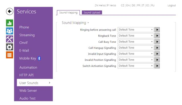
The **2N Helios IP** intercoms provide standard signalling of operational statuses by tone sequences; refer to the Signalling of Operational Statuses subsection. If you find the standard sound signalling inconvenient, modify the sounds for the following statuses:
