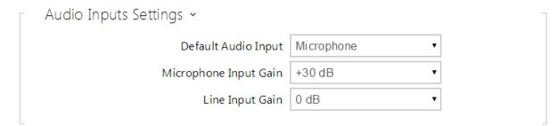
• **Default audio input** – set the default audio input (microphone, line input or audio module input) to be used for phone calls and audio streaming.
