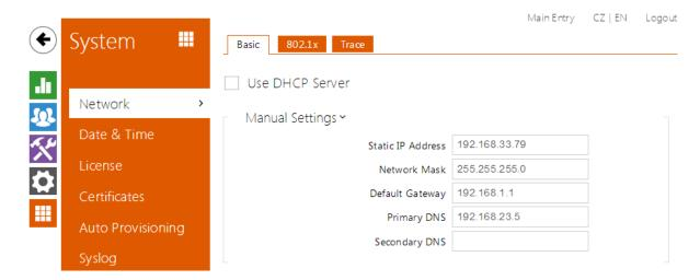
As the **2N Helios IP** intercom is connected to the LAN, make sure that its IP address has been set correctly or obtained from the LAN DHCP server. Configure the IP address and DHCP in the **Network** subsection.
