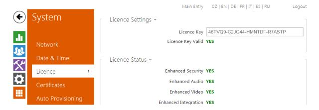
Some 2N Helios IP functions are available with a valid licence key only. Refer to the Model Differences and Function Licensing subsection for the list of intercom licensing options.
