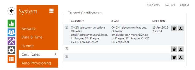
Some 2N Helios IP network services use the Transaction Layer Security (TLS) protocol for communication with other LAN devices to prevent third parties from monitoring and/or modifying the communication contents. Unilateral or bilateral authentication based on certificates and private keys is needed for establishing connections via TLS.
