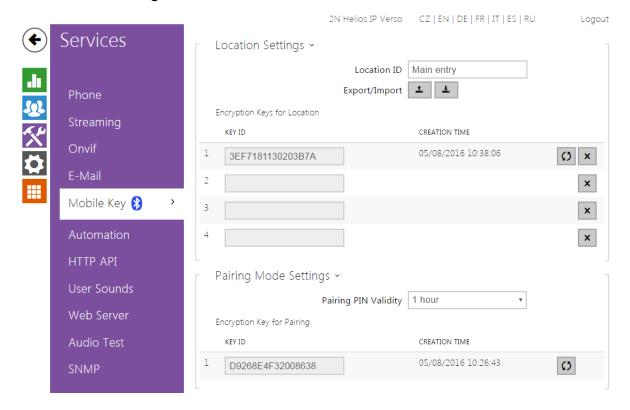
The **2N** Helios IP intercoms equipped with the Bluetooth module allow for user authentication via the **2N** Mobile Key application available to devices with iOS 8.1 and higher (iPhone 4s and higher phones) or Android 4.4 KitKat and higher (Bluetooth 4.0 Smart supporting phones).
