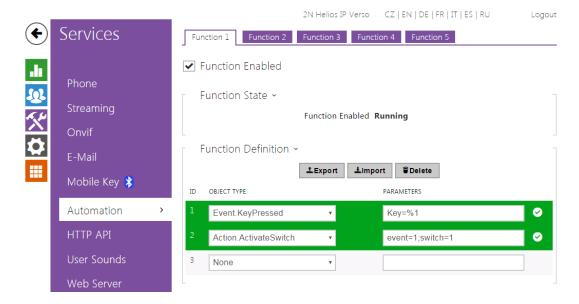
The **2N Helios IP** intercom provides highly flexible setting options to satisfy variable user needs. There are situations in which the standard configuration settings (switch or call modes, e.g.) are insufficient and so **2N Helios IP** offers **Automation**, a special programmable interface for applications that require complex interconnections with third party systems.
