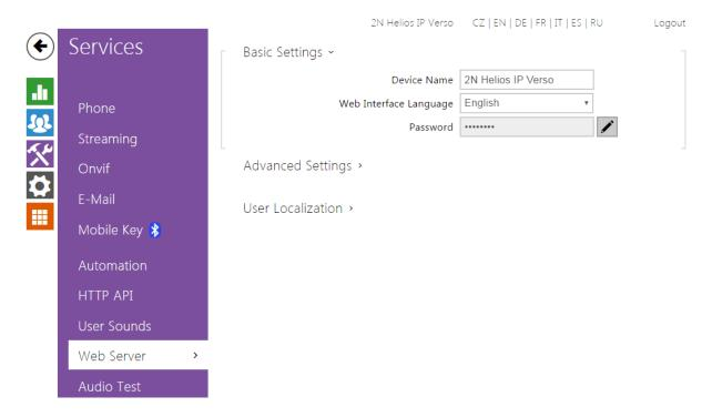
You can configure your **2N** Helios IP intercom using a standard browser which accesses the integrated web server. Use the secured HTTPS protocol for communication between the browser and intercom. Having accessed the intercom, enter the login name and password. The default login name and password are **admin** and **2n** respectively. We recommend you to change the default password as soon as possible.
