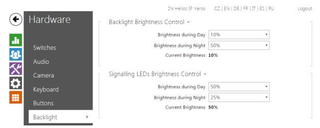
This tab helps you control the backlight level of nametags, buttons and brightness of signalling LEDs.
