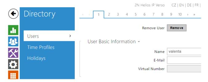
The Users list is one of the crucial parts of the intercom configuration. It contains user information relevant for such intercom functions as quick dialling, RFID card/code door unlocking, missed call e-mails and so on.
