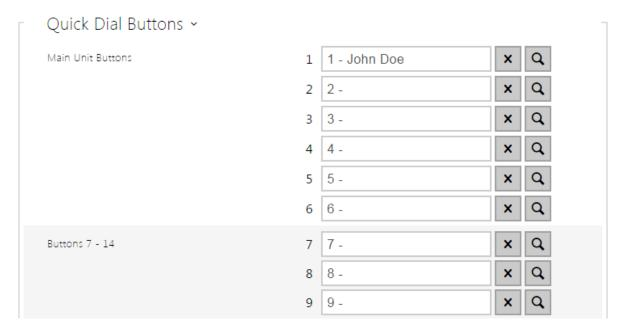
Display the list of all potentially available intercom buttons including those that are physically absent. In some intercom models ( $2N^{\text{@}}$  Helios IP Vario,  $2N^{\text{@}}$  Helios IP Verso), the button list is divided into 8/5-item groups corresponding to the button extending modules. Enter the user list position number or click  $\bigcirc$  to search a user by the name easily.
