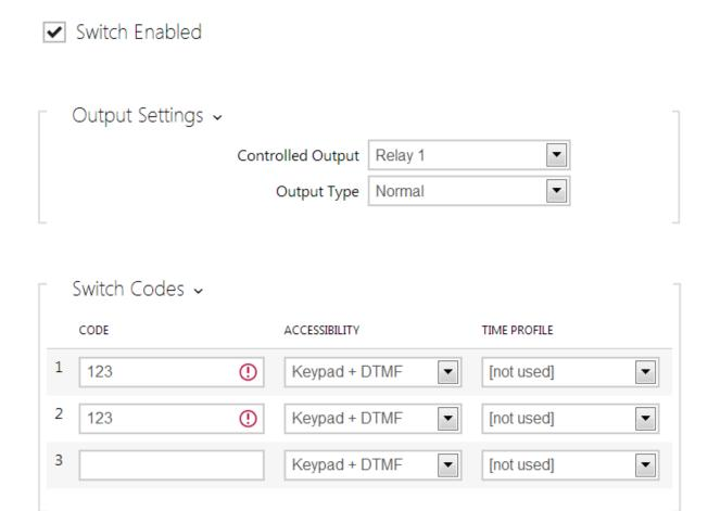
Enable the switch in the **Switch Enabled** parameter in the **Hardware / Switches / Switch 1** tab, set the **Controlled Output** to the intercom output to which the electric door lock is connected. Now set one or more activation codes for the electric door lock switching.
