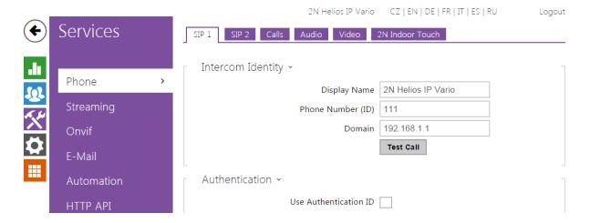
The Phone service is one of the basic functions of the intercom: helps you establish connections with other IP network terminal equipment. The **2N Helios IP** intercoms support the extended SIP and are compatible with and certified by the leading SIP PBX and terminal equipment manufacturers (CISCO, Avaya, Broadsoft, etc.).
