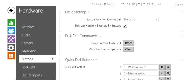
Assign the **Directory** / **Users** users to the quick dial buttons. By default, all available intercom buttons are assigned to the listed users. A non-assigned button can be used for automation or switch activation, for example.
