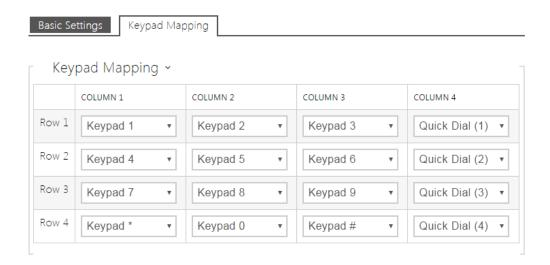
You can assign one function to each matrix position: numeric keypad keys 0 through 9, \*, # or one of the quick dial buttons 1-16.
