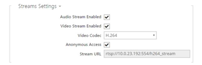
• Audio stream enabled - enable offering of audio stream while establishing connection with the RTSP server.
