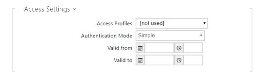
Each user is assigned an access mode for intercom authentication.
