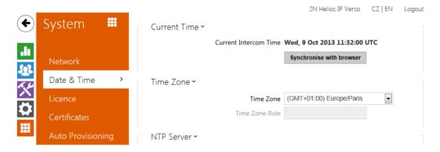
If you control validity of phone numbers, lock activation codes and similar by time profiles, make sure that the intercom internal date and time are set correctly.
