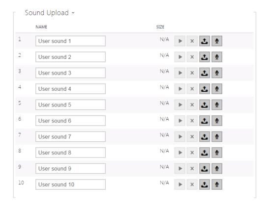
You can record a sound file using your PC microphone. Press • to start the record and press • to stop the record. Press • to play the sound record. Click **Upload** to save the sound into the intercom.
