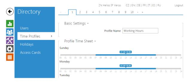
Such intercom functions as outgoing calls and RFID card/numeric code access, for example, can be time-limited by being assigned a **time profile**. By assigning a time profile you can:
