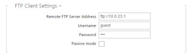
• Remote FTP server address - set the FTP server address in the ftp://ip\_address or ftps://ip\_address format.
