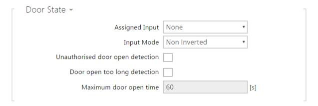
The models equipped with one digital input at least help connect an open door sensor and signal any unauthorised door opening or door closing failure with a timeout. The events are written into a log and read out using HTTP API (refer to the 2N <sup>®</sup> Helios IP HTTP API manual). This function is available only for Switch 1.
