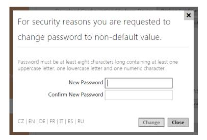
Remember the new password well or put it down just in case. Because if you forget the password, you will have to reset the intercom to default values (refer to the Installation Manual of your intercom model) and lose all your current configuration changes.
