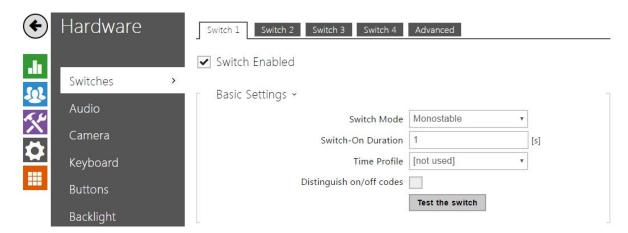
Switches provide a very flexible and efficient control of such intercom peripherals as electric door locks, lighting, additional ringing signalling, and so on. **2N Helios IP** allows you to configure up to 4 (depending on model types) independent all-purpose switches.
